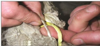
Fig. 1 Inspect for Internal Abrasion.
